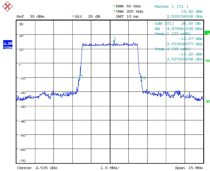
**LTE band 7, 5MHz Bandwidth,16QAM (-26dBc BW)**
