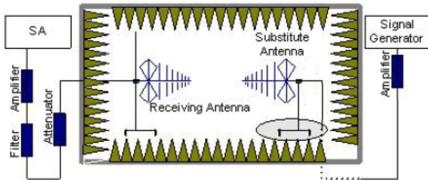
In the chamber, a substitution antenna for the frequency band of interest is placed at the reference point of the chamber. An RF signal source for the frequency band of interest is
