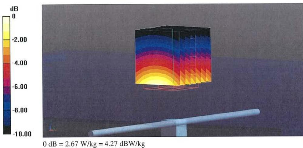
Impedance Measurement Plot for Head TSL
