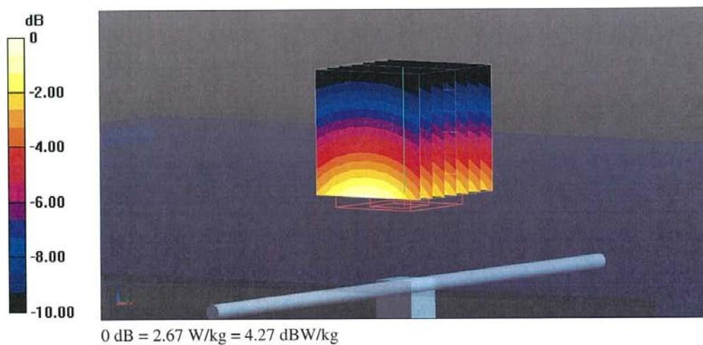
Impedance Measurement Plot for Head TSL
