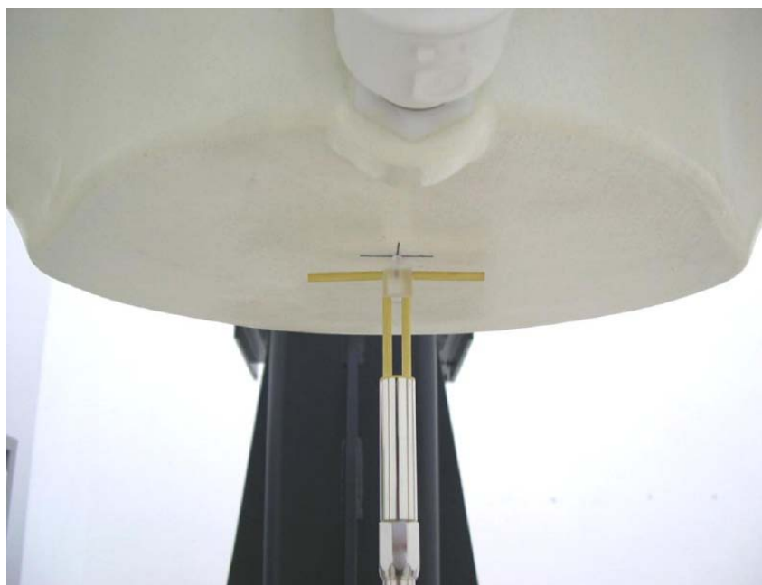
Picture 8.2 Photo of Dipole Setup
