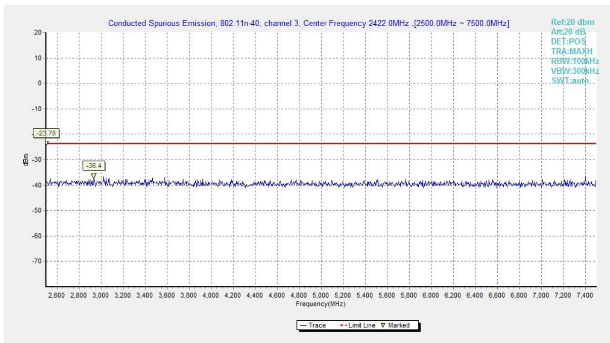
Fig.A.6.1.76 Transmitter Spurious Emission - Conducted (802.11n-HT40, Ch3, 2.5 GHz-7.5 GHz)
