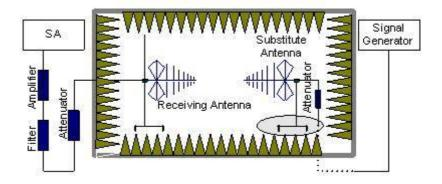
In the chamber, an substitution antenna for the frequency band of interest is placed at the reference point of the chamber. An RF Signal source for the frequency band of interest is connected to the substitution antenna with a cable that has been constructed to not interfere with the radiation pattern of the antenna. A power  $(P_{Mea})$  is applied to the input of the
