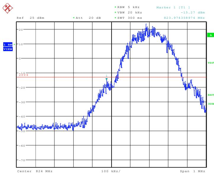
**HIGH BAND EDGE BLOCK-C (GSM850) –Channel 251**
