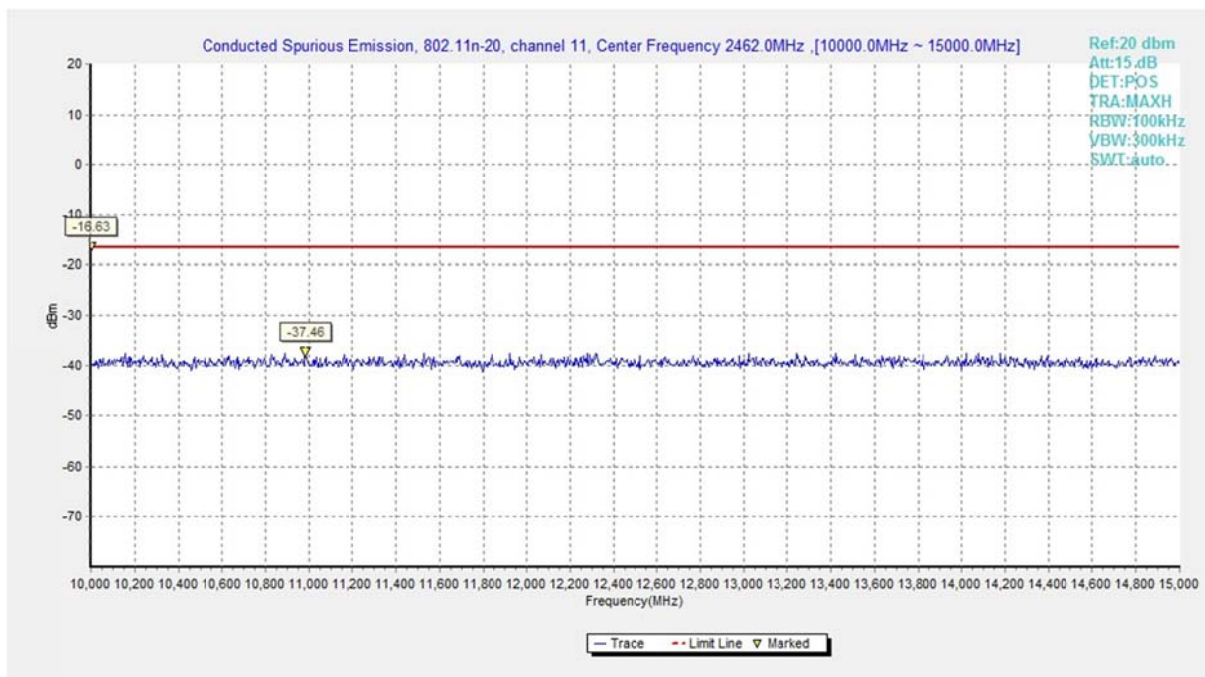
Fig.A.6.1.70 Transmitter Spurious Emission - Conducted (802.11n-HT20, Ch11, 10 GHz-15 GHz)
