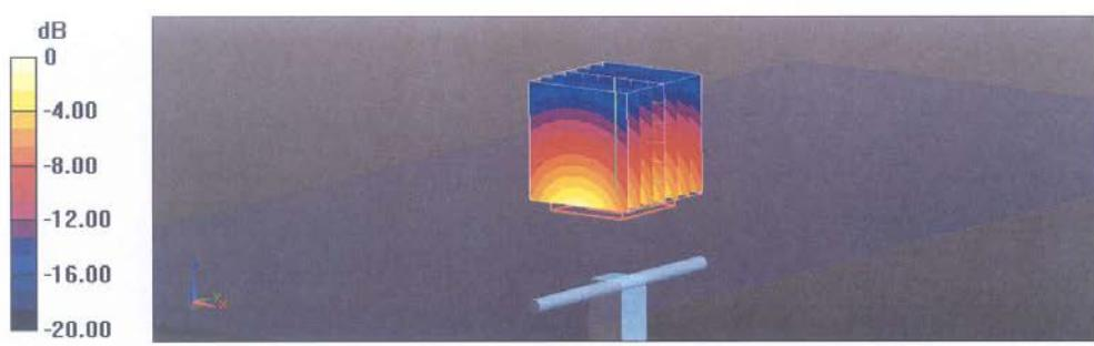
Impedance Measurement Plot for Head TSL
