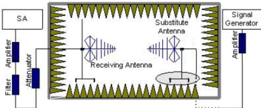
In the chamber, an substitution antenna for the frequency band of interest is placed at the reference point of the chamber. An RF Signal source for the frequency band of interest is connected to the substitution antenna with a cable that has been constructed to not interfere
