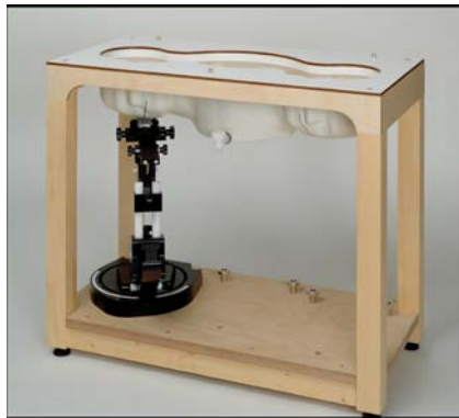
Picture C.10: SAM Twin Phantom
