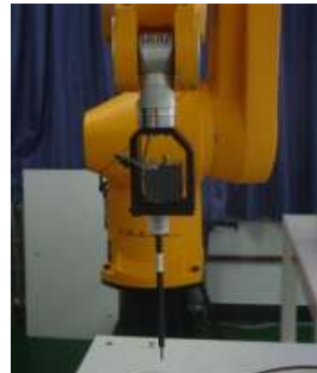
Picture C.3 E-field Probe
