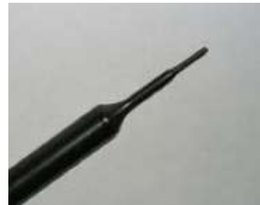
Picture C.2 Near-field Probe
