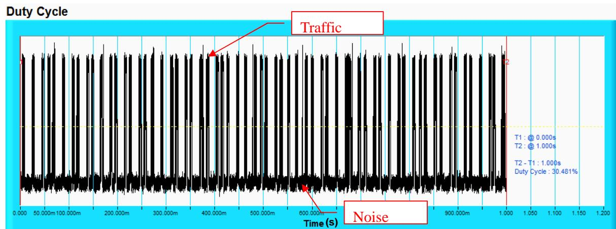
**NOTE:** T1 denotes the start of duty cycle period is 0th second. T2 denotes the end of duty cycle period is 1th second. T2 – T1= 1 seconds. Duty Cycle = 30.481%.
