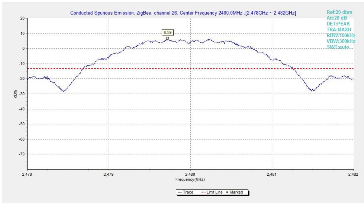
Fig.A.6.1.17 Transmitter Spurious Emission - Conducted (Zigbee Channel 26, Center Frequency)
