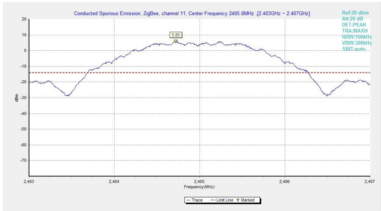
Fig.A.6.1.1 Transmitter Spurious Emission - Conducted (Zigbee Channel 11, Center Frequency)
