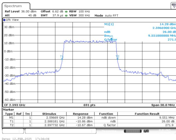
**LTE band 41 , 10MHz Bandwidth,MID,16QAM (-26dBc BW)**
