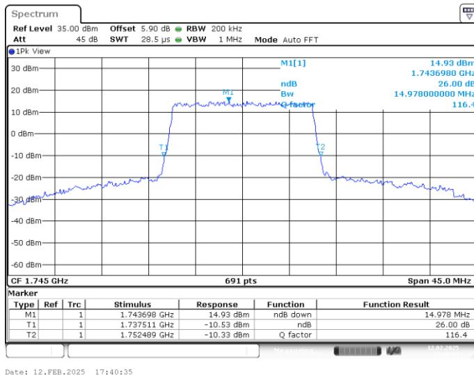
**LTE band 66 , 15MHz Bandwidth,MID,16QAM (-26dBc BW)**
