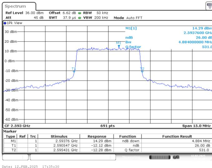
**LTE band 41 , 5MHz Bandwidth,MID,16QAM (-26dBc BW)**
