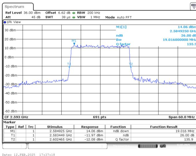
**LTE band 41 , 20MHz Bandwidth,MID,16QAM (-26dBc BW)**
