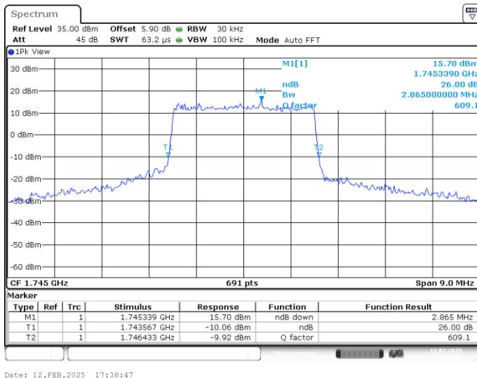
**LTE band 66 , 3MHz Bandwidth,MID,16QAM (-26dBc BW)**
