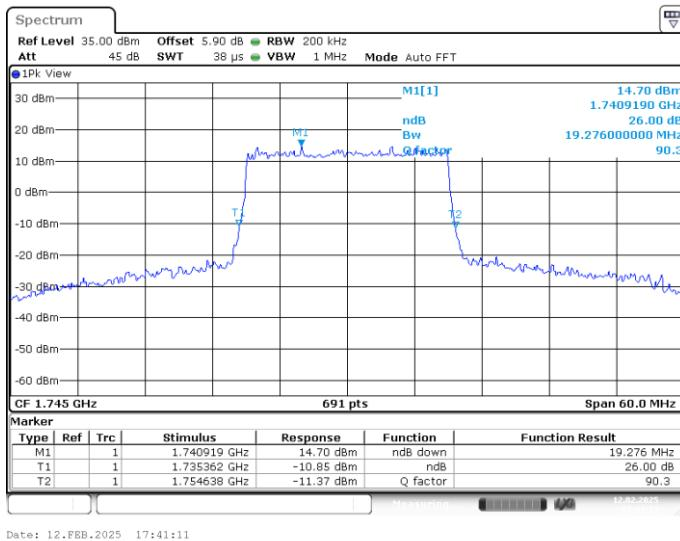
**LTE band 66 , 20MHz Bandwidth,MID,16QAM (-26dBc BW)**
