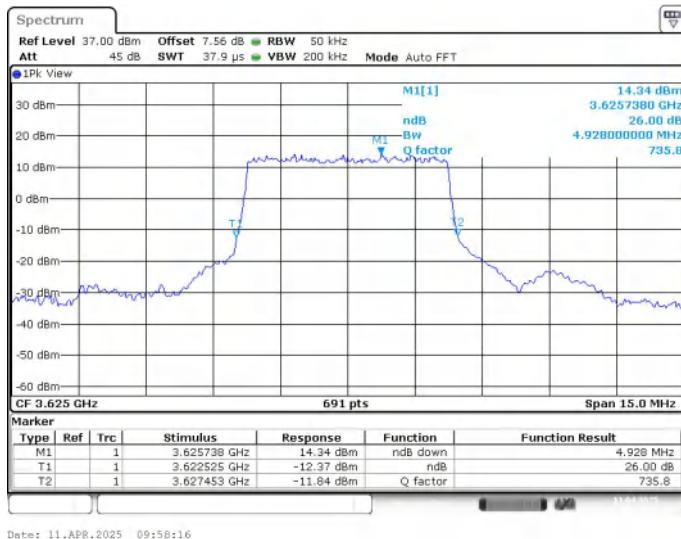
**LTE band 48 , 5MHz Bandwidth,MID,16QAM (-26dBc BW)**
