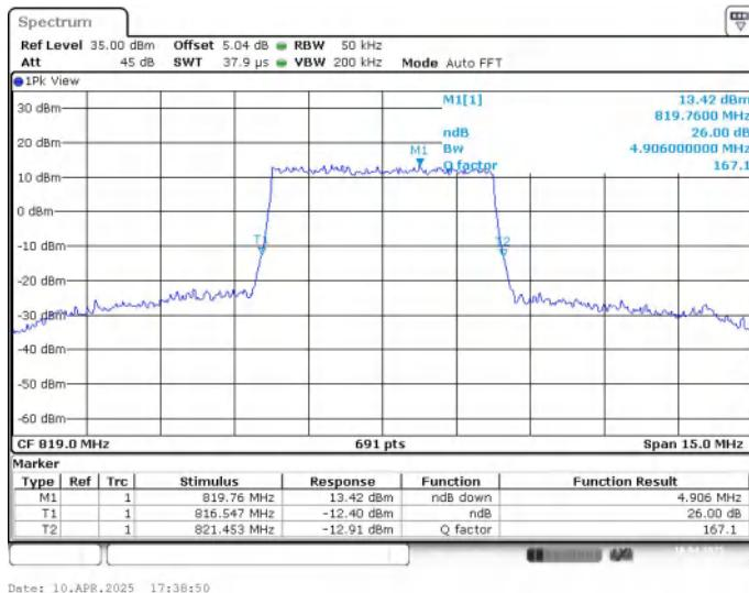
**LTE band 26 , 5MHz Bandwidth,MID,16QAM (-26dBc BW)**
