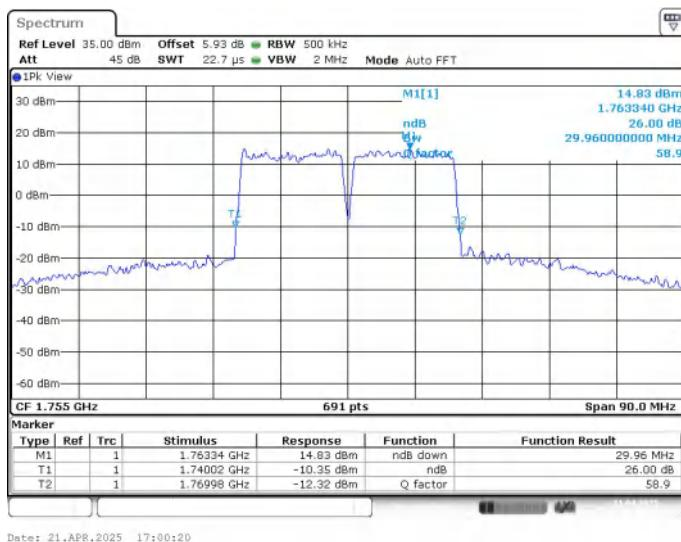
**LTE CA band 66C , 15MHz+15MHz Bandwidth,16QAM (-26dBc BW)**
