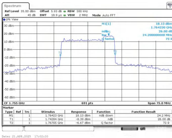
**LTE CA band 66C , 20MHz+5MHz Bandwidth,16QAM (-26dBc BW)**
