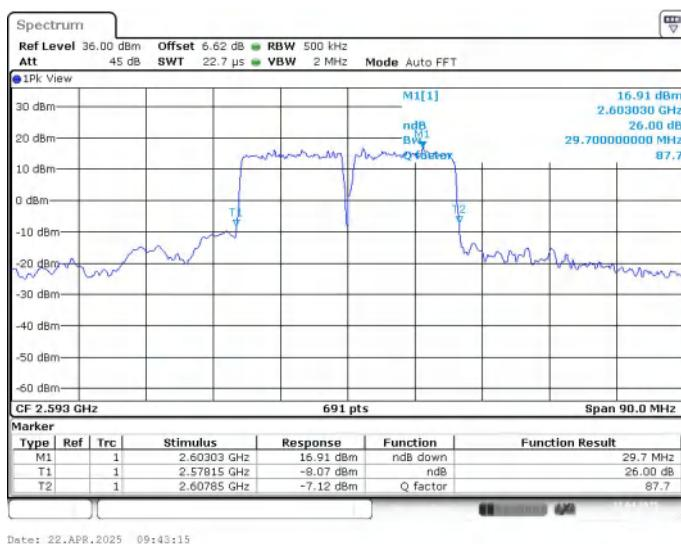
**LTE CA band 41C , 15MHz+15MHz Bandwidth,16QAM (-26dBc BW)**
