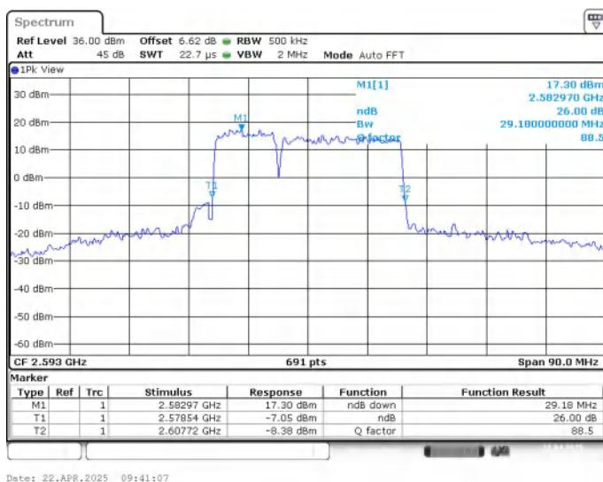
**LTE CA band 41C , 10MHz+20MHz Bandwidth,16QAM (-26dBc BW)**
