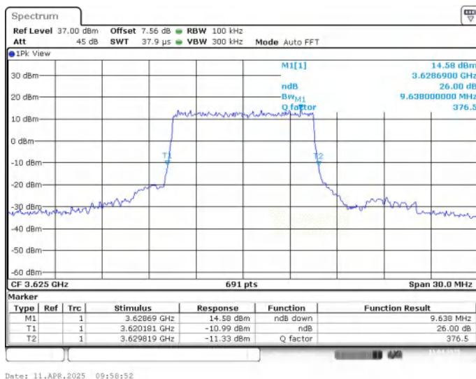
**LTE band 48 , 10MHz Bandwidth,MID,16QAM (-26dBc BW)**
