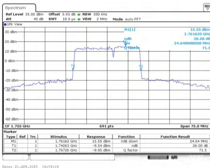
**LTE CA band 66C , 15MHz+10MHz Bandwidth,16QAM (-26dBc BW)**
