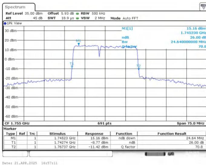
**LTE CA band 66C , 10MHz+15MHz Bandwidth,16QAM (-26dBc BW)**
