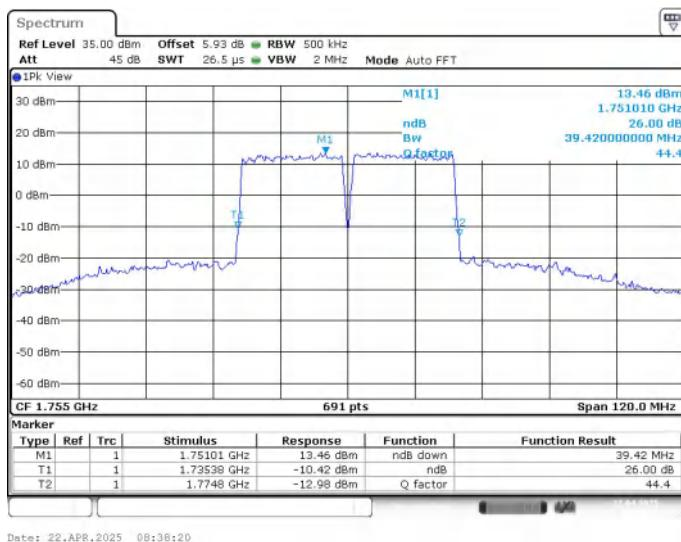
**LTE CA band 66C , 20MHz+20MHz Bandwidth,16QAM (-26dBc BW)**
