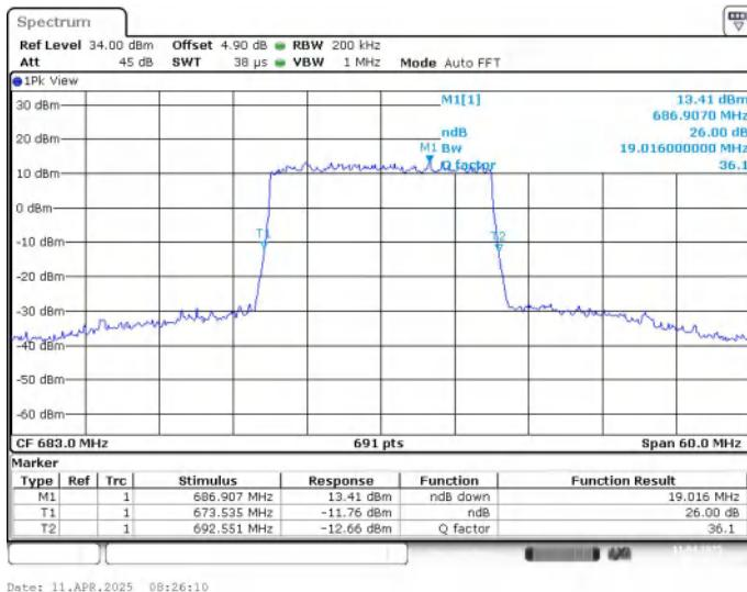
**LTE band 71 , 20MHz Bandwidth,MID,16QAM (-26dBc BW)**
