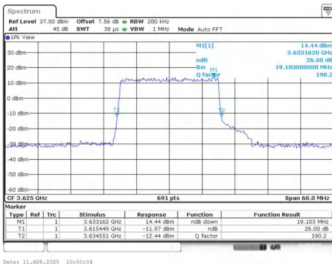
**LTE band 48 , 20MHz Bandwidth,MID,16QAM (-26dBc BW)**
