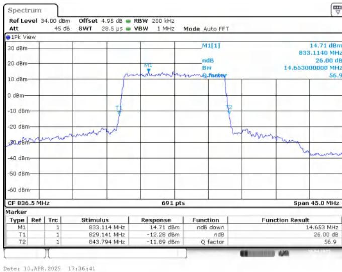
**LTE band 26 , 15MHz Bandwidth,MID,16QAM (-26dBc BW)**
