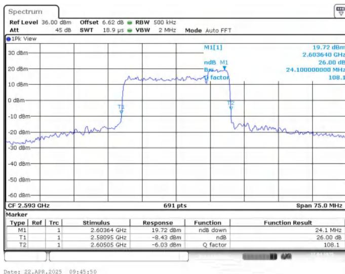
**LTE CA band 41C , 20MHz+5MHz Bandwidth,16QAM (-26dBc BW)**
