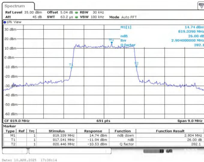
**LTE band 26 , 3MHz Bandwidth,MID,16QAM (-26dBc BW)**
