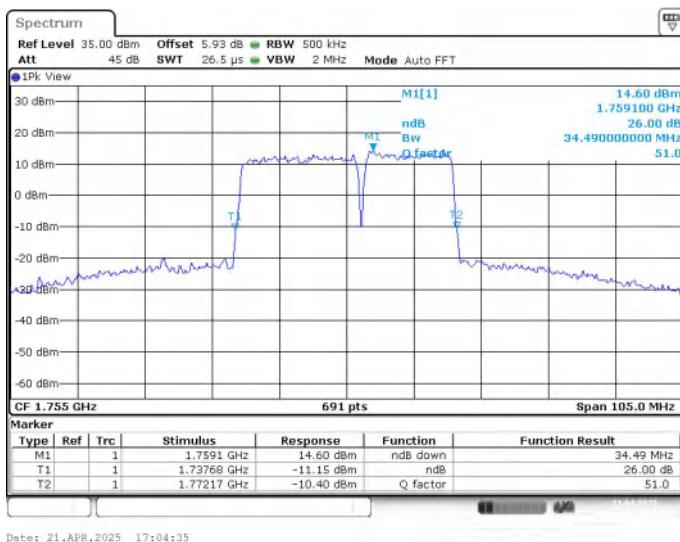
**LTE CA band 66C , 20MHz+15MHz Bandwidth,16QAM (-26dBc BW)**
