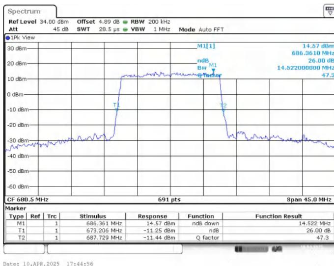
**LTE band 71 , 15MHz Bandwidth,MID,16QAM (-26dBc BW)**
