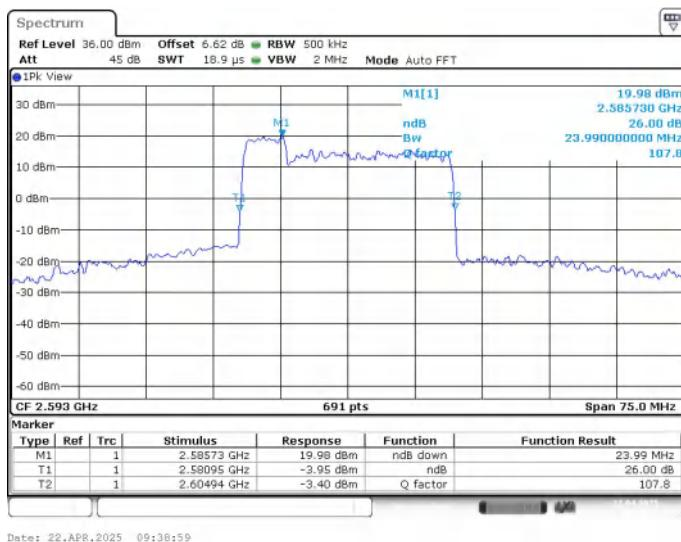
**LTE CA band 41C , 5MHz+20MHz Bandwidth,16QAM (-26dBc BW)**
