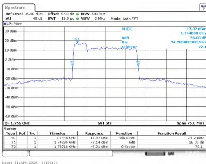
**LTE CA band 66C , 5MHz+20MHz Bandwidth,16QAM (-26dBc BW)**
