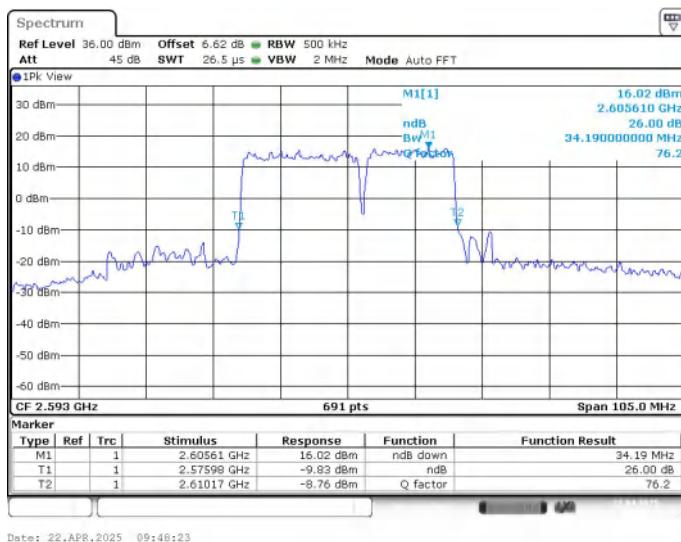
**LTE CA band 41C , 20MHz+15MHz Bandwidth,16QAM (-26dBc BW)**
