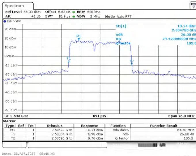
**LTE CA band 41C , 10MHz+15MHz Bandwidth,16QAM (-26dBc BW)**
