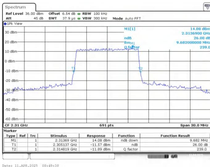
**LTE band 30 , 10MHz Bandwidth,MID,16QAM (-26dBc BW)**
