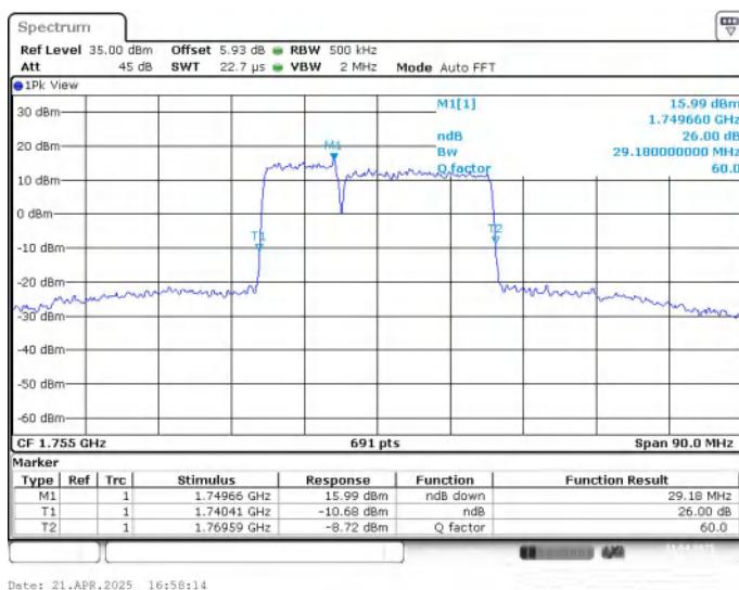
**LTE CA band 66C , 10MHz+20MHz Bandwidth,16QAM (-26dBc BW)**
