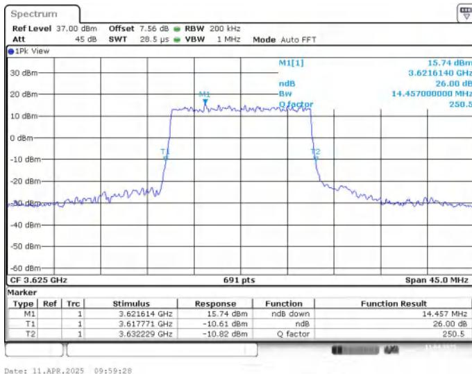
**LTE band 48 , 15MHz Bandwidth,MID,16QAM (-26dBc BW)**
