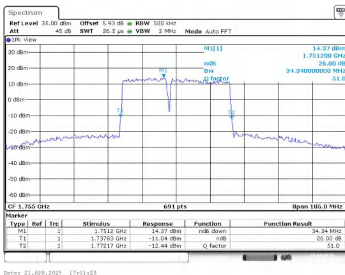
**LTE CA band 66C , 15MHz+20MHz Bandwidth,16QAM (-26dBc BW)**
