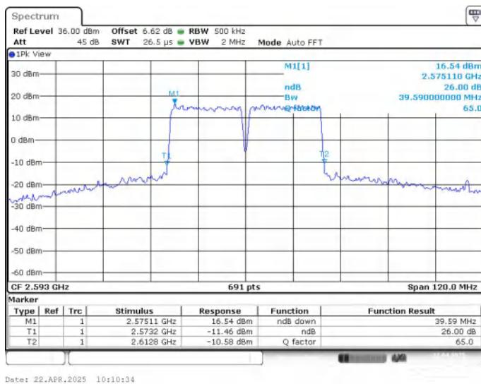
**LTE CA band 41C , 20MHz+20MHz Bandwidth,16QAM (-26dBc BW)**
