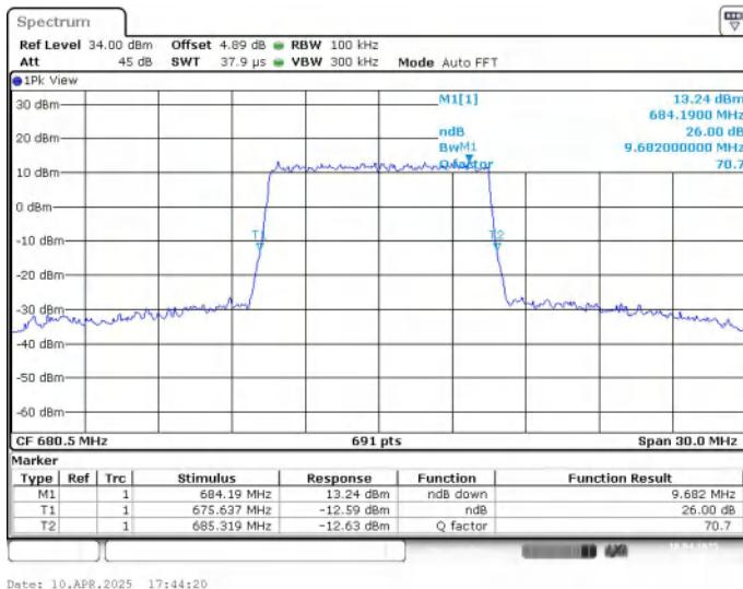
**LTE band 71 , 10MHz Bandwidth,MID,16QAM (-26dBc BW)**
