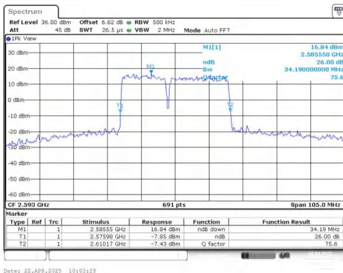
**LTE CA band 41C , 15MHz+20MHz Bandwidth,16QAM (-26dBc BW)**
