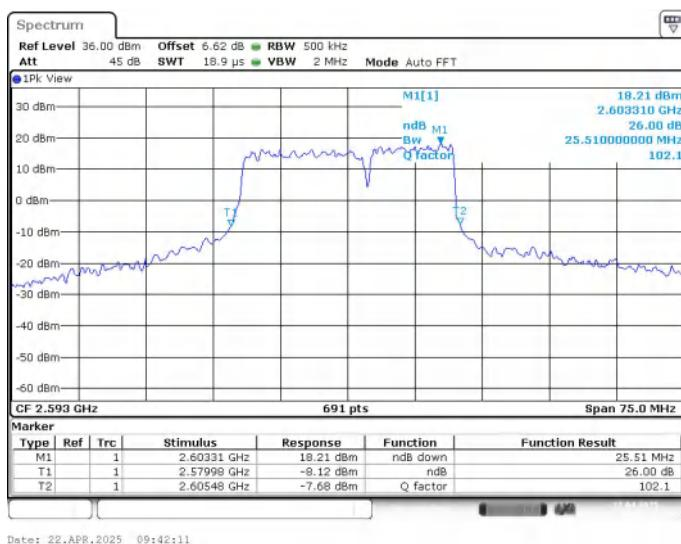
**LTE CA band 41C , 15MHz+10MHz Bandwidth,16QAM (-26dBc BW)**
