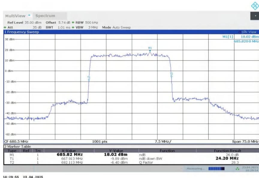
n71,25MHz Bandwidth,DFT-s-QPSK (-26dBc BW)
