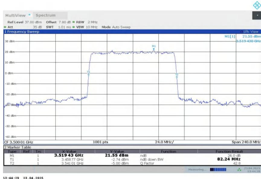
**n77L,80MHz Bandwidth,DFT-s-QPSK (-26dBc BW)**
