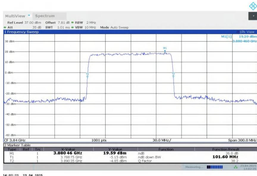
**n77H,100MHz Bandwidth,DFT-s-16QAM (-26dBc BW)**
