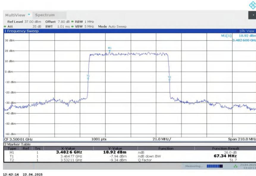
**n77L,70MHz Bandwidth,DFT-s-QPSK (-26dBc BW)**
