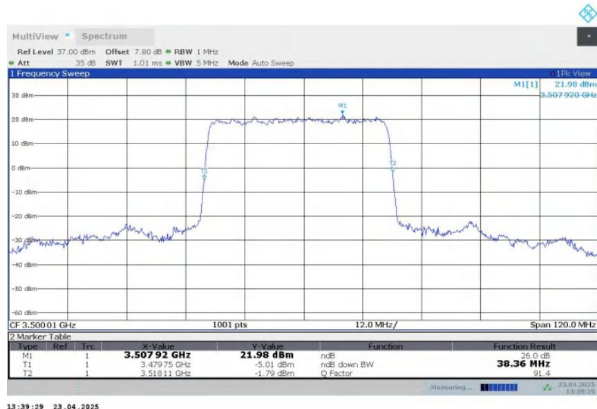
**n77L,40MHz Bandwidth,DFT-s-QPSK (-26dBc BW)**
