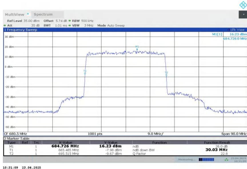
n71,30MHz Bandwidth,DFT-s-QPSK (-26dBc BW)
