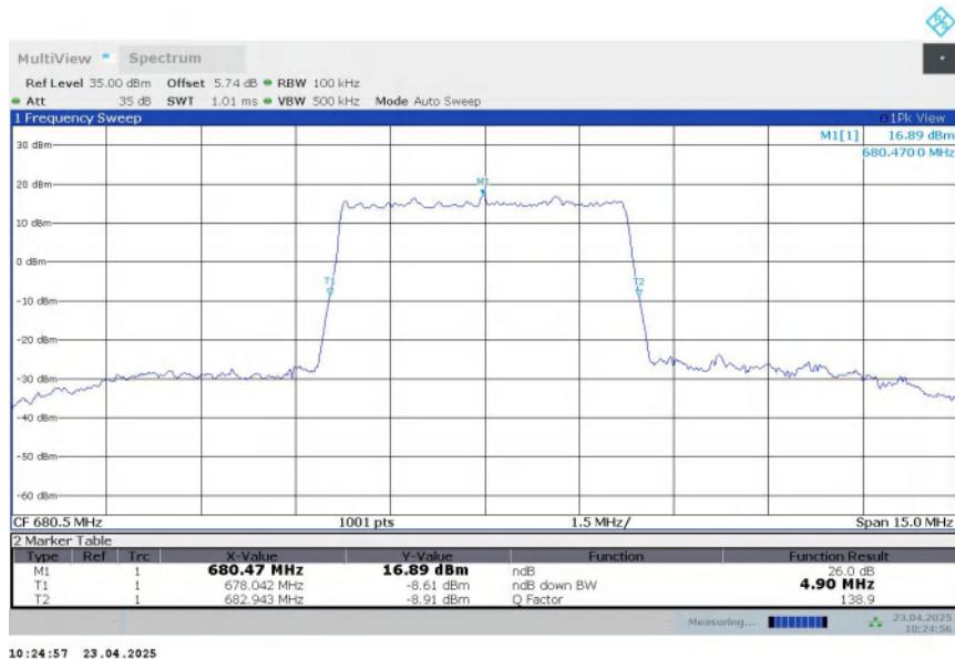
n71,5MHz Bandwidth,DFT-s-QPSK (-26dBc BW)
