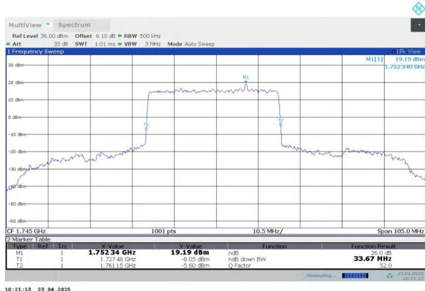
n66,35MHz Bandwidth,DFT-s-QPSK (-26dBc BW)
