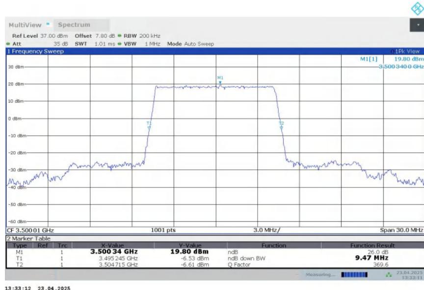
**n77L,10MHz Bandwidth,DFT-s-QPSK (-26dBc BW)**
