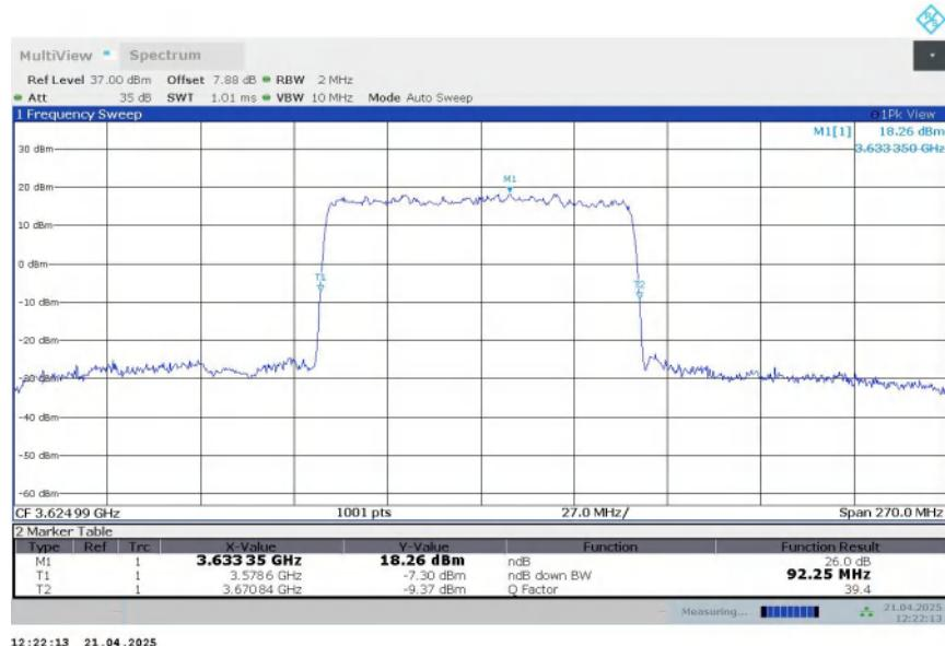
n48,90MHz Bandwidth,DFT-s-QPSK (-26dBc BW)
