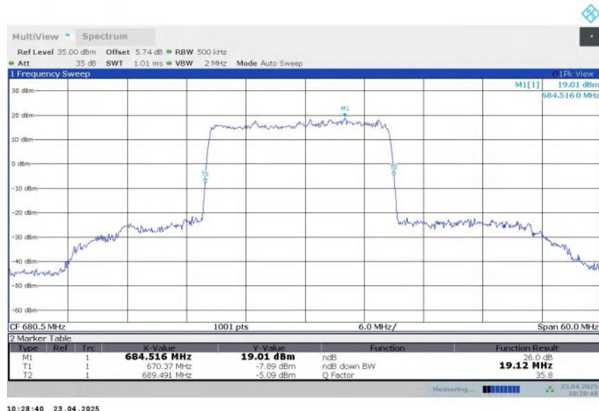
n71,20MHz Bandwidth,DFT-s-QPSK (-26dBc BW)
