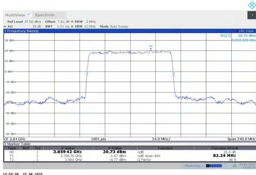
**n77H,80MHz Bandwidth,DFT-s-QPSK (-26dBc BW)**
