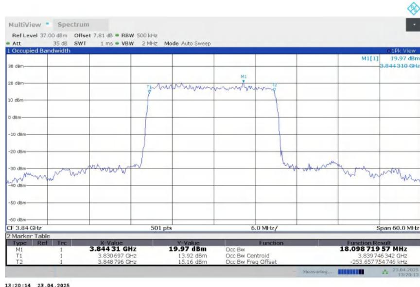
**n77H,20MHz Bandwidth,DFT-s-QPSK (99% BW)**
