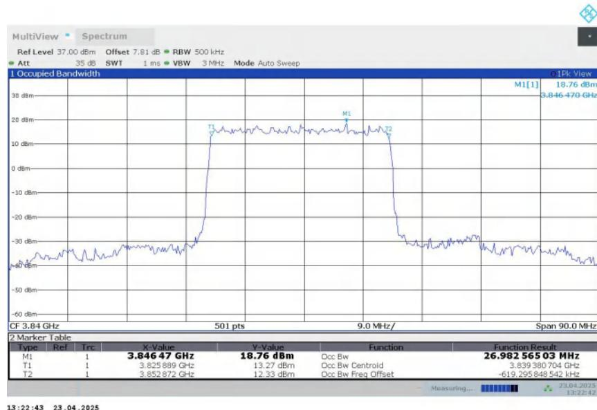
**n77H,30MHz Bandwidth,DFT-s-QPSK (99% BW)**
