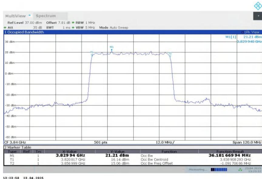
**n77H,40MHz Bandwidth,DFT-s-QPSK (99% BW)**
