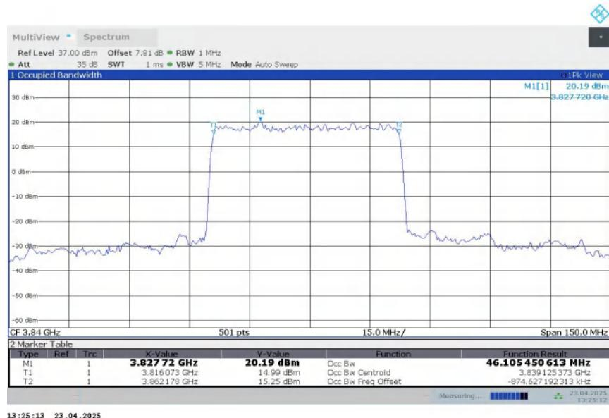
**n77H,50MHz Bandwidth,DFT-s-QPSK (99% BW)**
