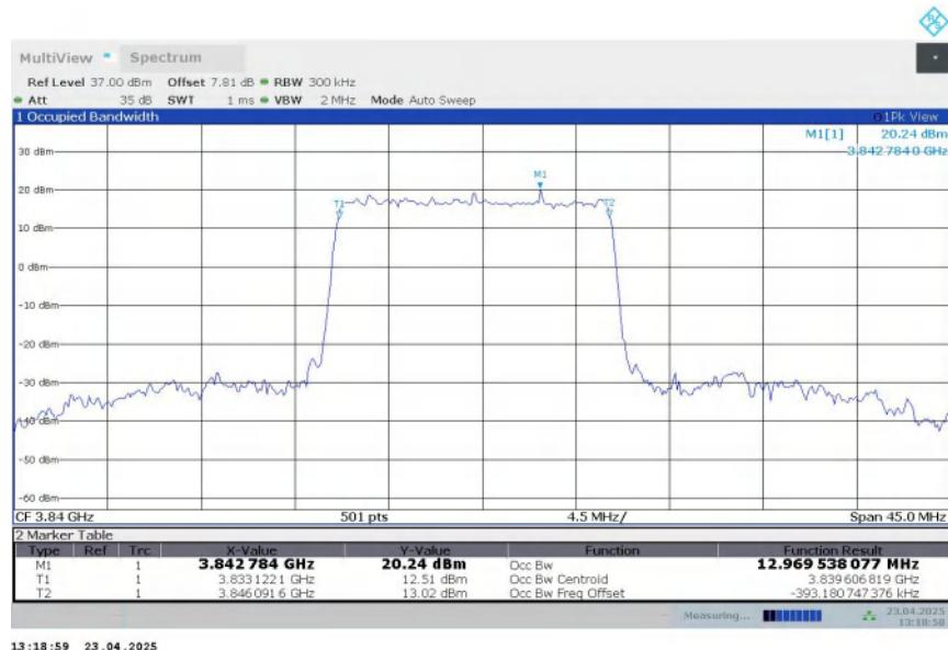
**n77H,15MHz Bandwidth,DFT-s-QPSK (99% BW)**
