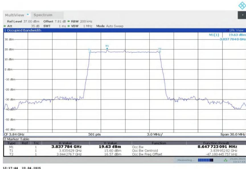
**n77H,10MHz Bandwidth,DFT-s-QPSK (99% BW)**
