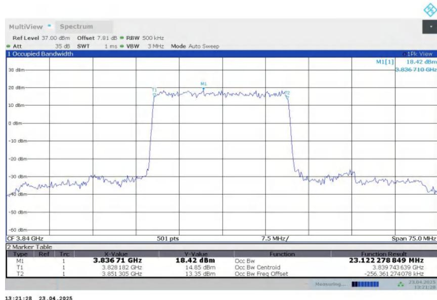
**n77H,25MHz Bandwidth,DFT-s-QPSK (99% BW)**
