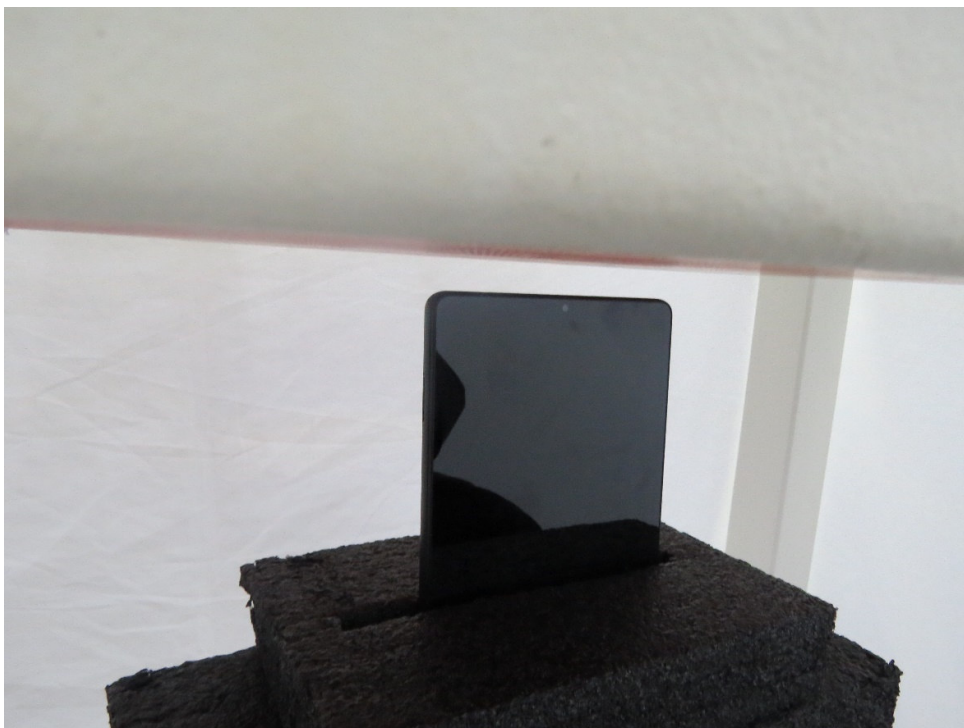
Picture 11: Top Edge, the distance from EUT to the bottom of the Phantom is 14mm
