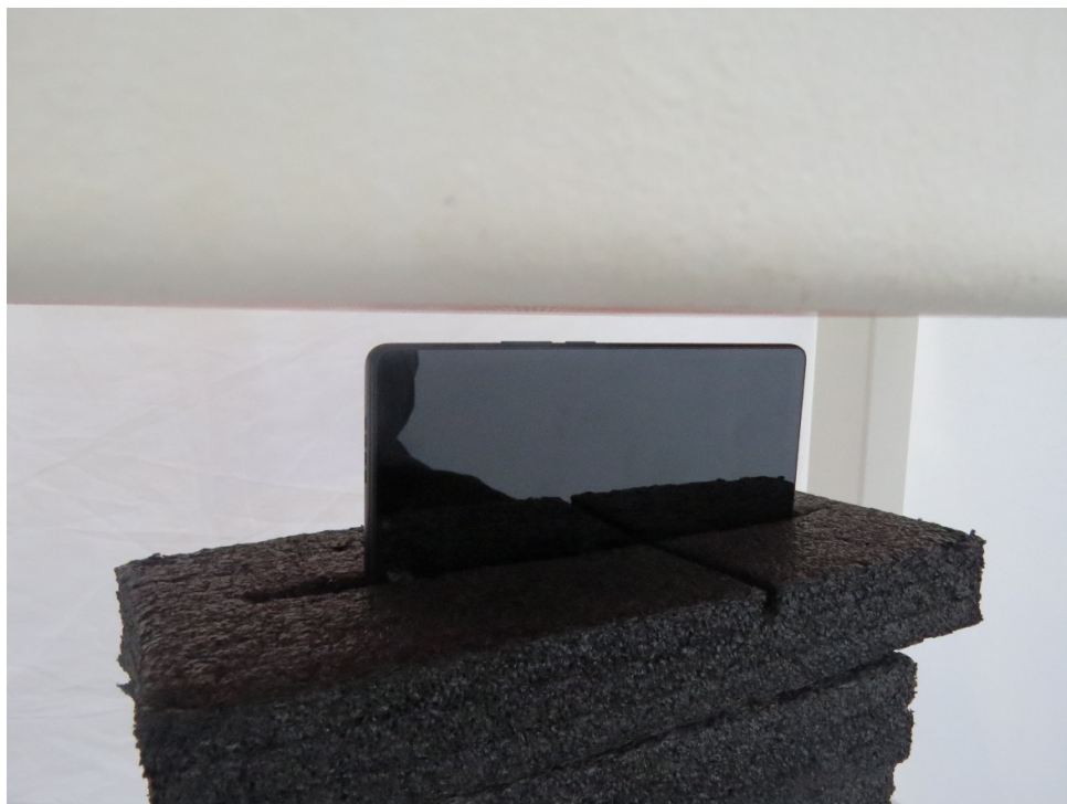
Picture 9: Right Edge, the distance from EUT to the bottom of the Phantom is 13mm
