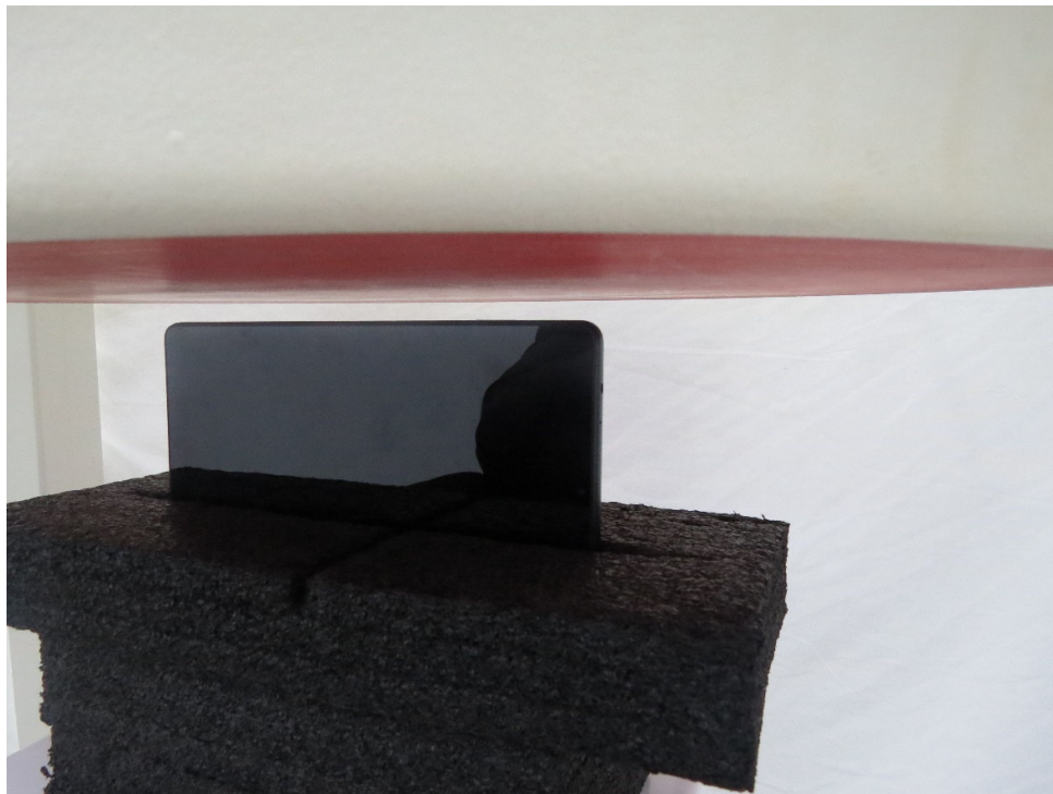
Picture 8: Left Edge, the distance from EUT to the bottom of the Phantom is 13mm
