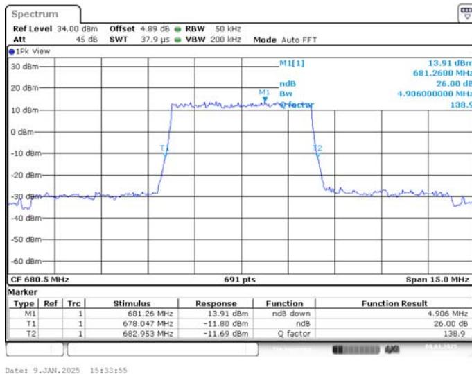
**LTE band 71 , 5MHz Bandwidth,MID,16QAM (-26dBc BW)**
