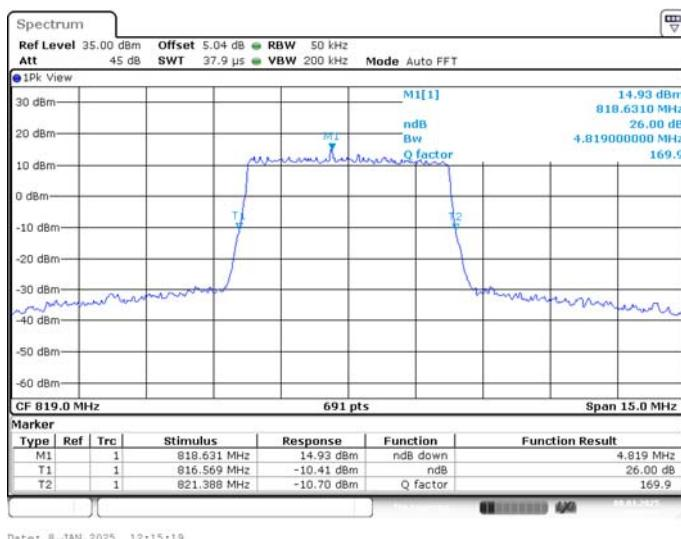
**LTE band 26(814MHz~824MHz),10MHz(-26dBc)**
