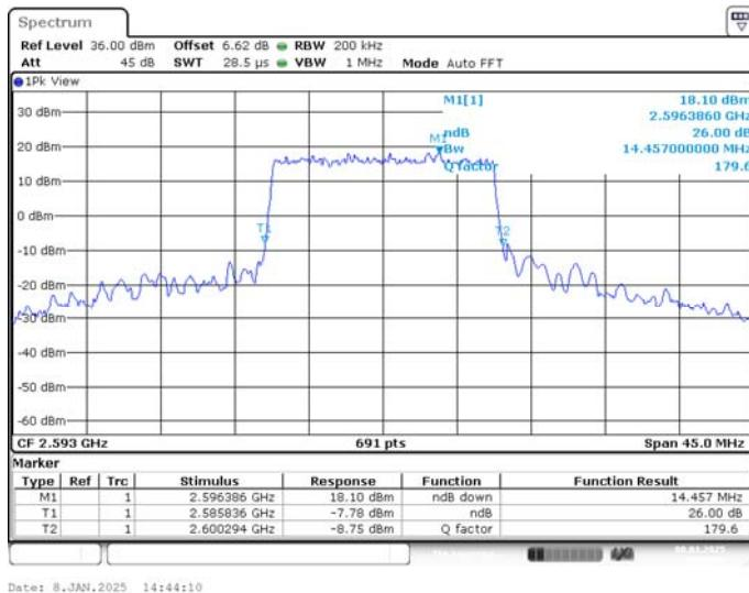
**LTE band 41 , 15MHz Bandwidth,MID,16QAM (-26dBc BW)**
