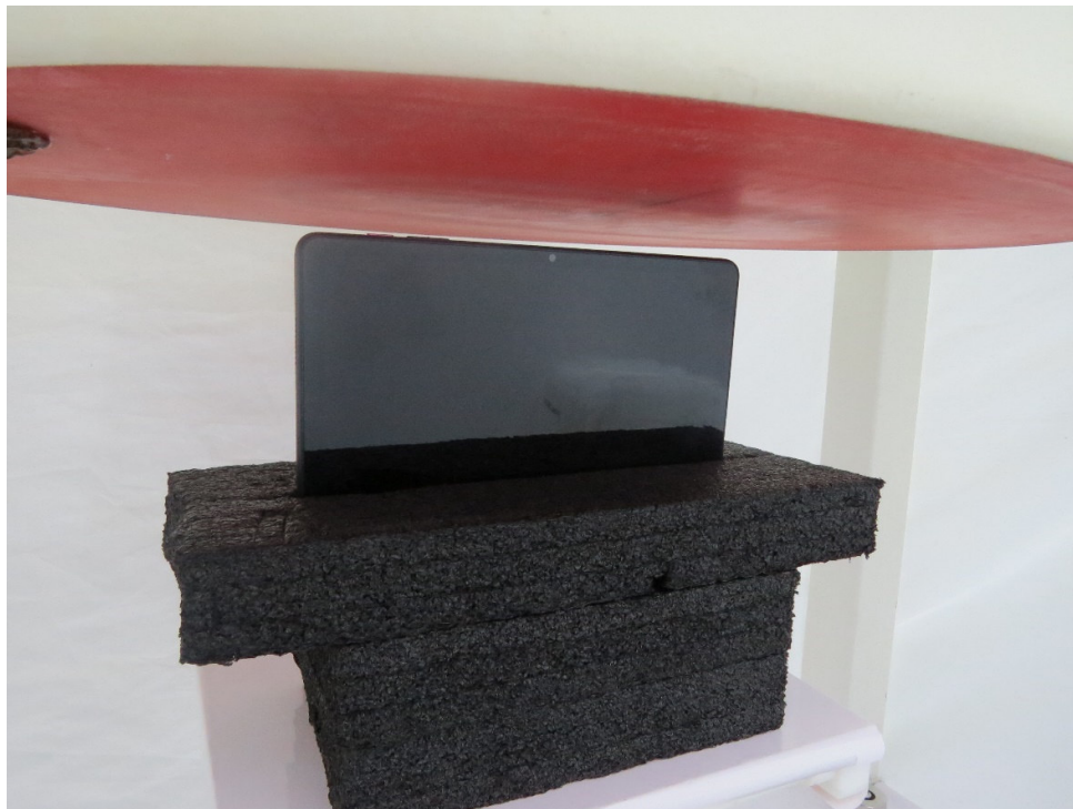
Picture 10: Top Edge, the distance from EUT to the bottom of the Phantom is 13mm
