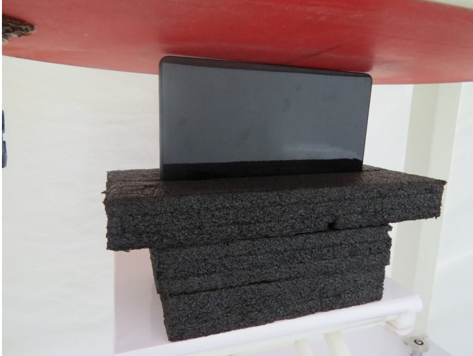
Picture 5: Bottom Edge, the distance from EUT to the bottom of the Phantom is 0mm
