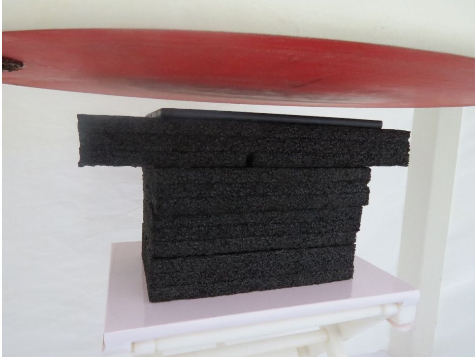
Picture 8: Back Side, the distance from EUT to the bottom of the Phantom is 24mm
