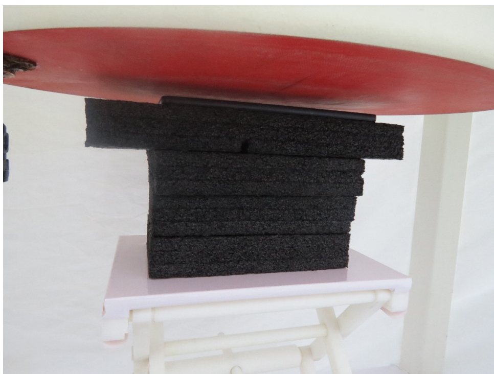
Picture 7: Back Side, the distance from EUT to the bottom of the Phantom is 14mm
