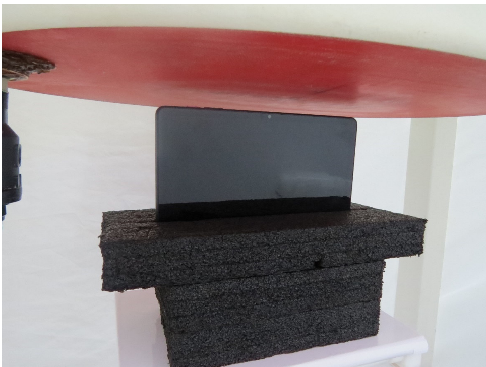
Picture 9: Top Edge, the distance from EUT to the bottom of the Phantom is 11mm
