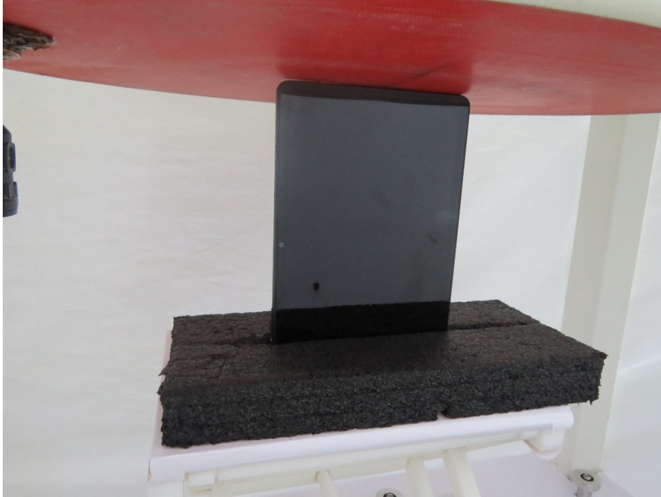
Picture 3: Right Edge, the distance from EUT to the bottom of the Phantom is 0mm
