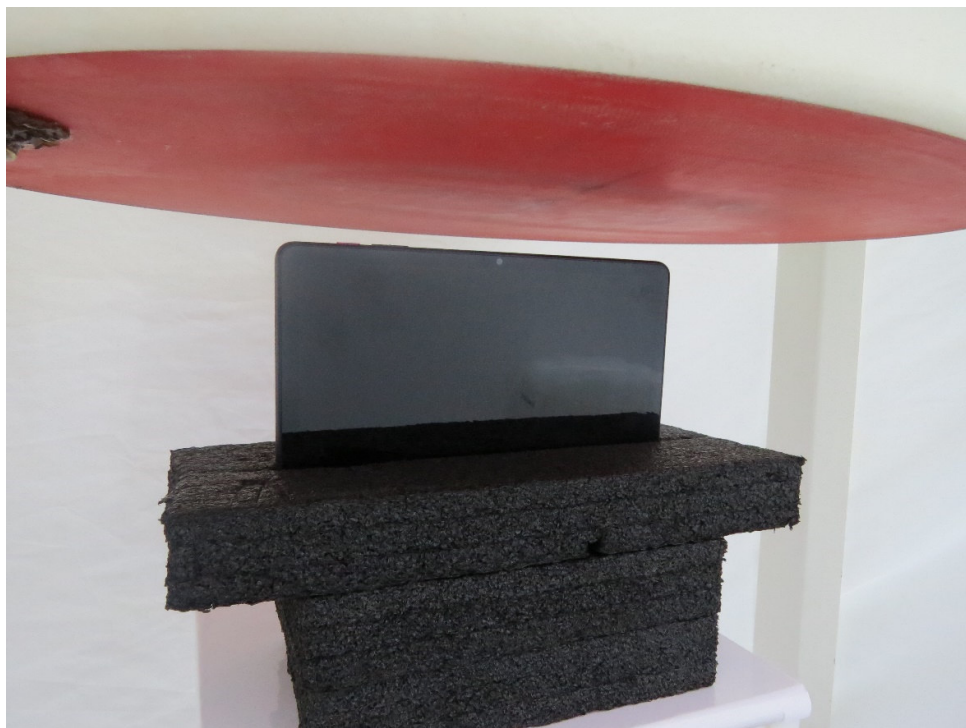
Picture 11: Top Edge, the distance from EUT to the bottom of the Phantom is 24mm
