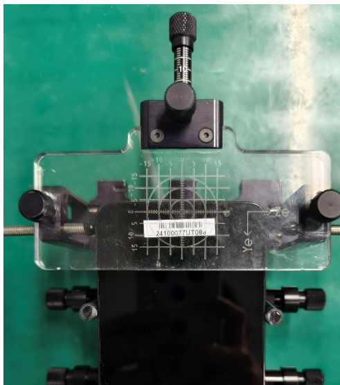
Pic 3: Handset Positioner (HHPIII) with mounted EUT mobile phone
