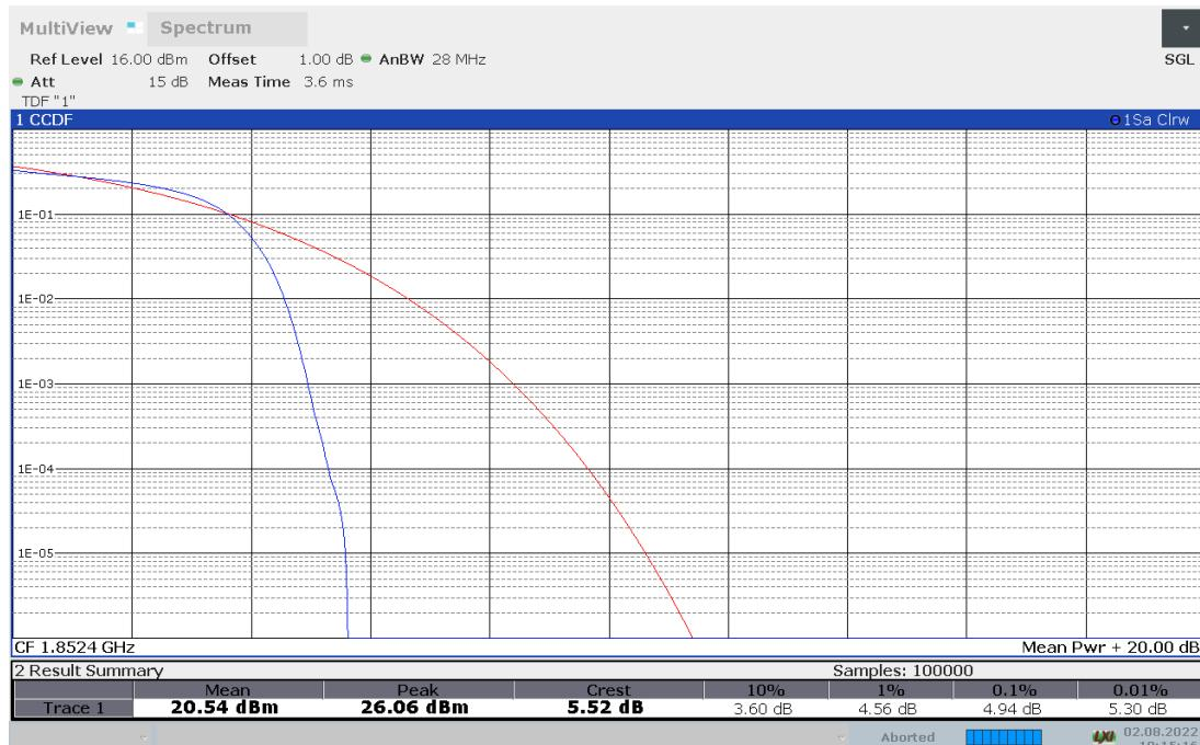
**Channel 9400- Peak-To-Average Power Ratio(PAPR)-16QAM**
