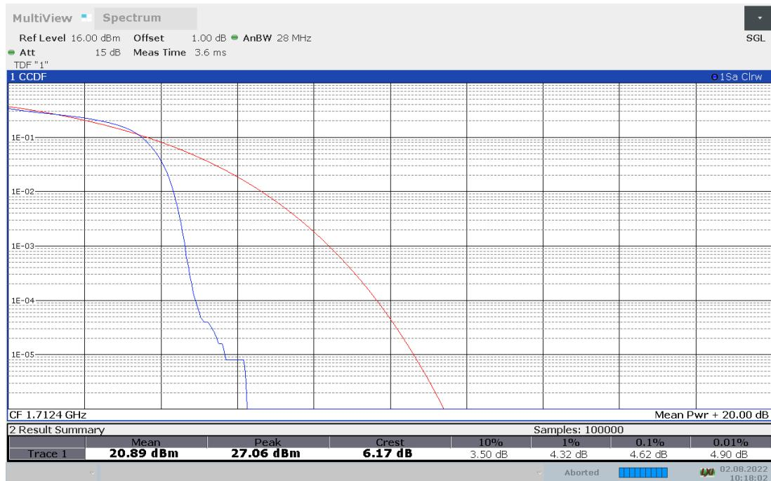
**Channel 1412- Peak-To-Average Power Ratio(PAPR)-16QAM**
