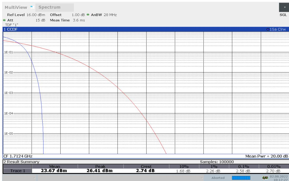
**Channel 1412- Peak-To-Average Power Ratio(PAPR)-QPSK**
