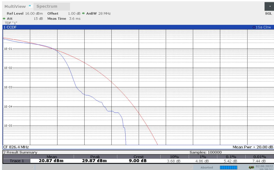
**Channel 4183- Peak-To-Average Power Ratio(PAPR)-16QAM**
