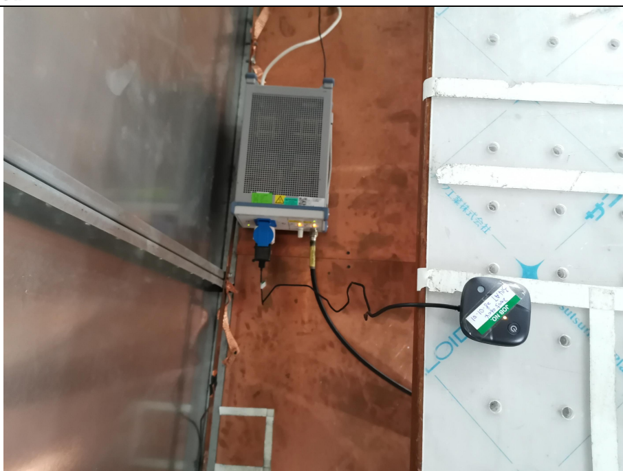
Conducted Emissions Test Setup (with charger)
