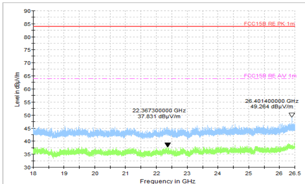
Figure A.1.3. Radiated Emission (GSM Receiver 850MHz,18GHz to 26.5GHz)
