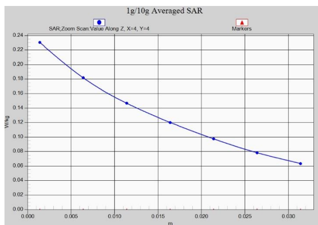
Z-Scan at power reference point (850 MHz)
