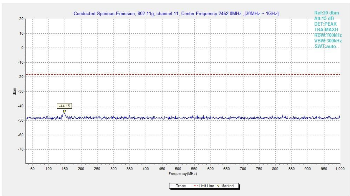
Fig.B.6.1.42 Transmitter Spurious Emission - Conducted (802.11g, Ch11, 30 MHz-1 GHz)
