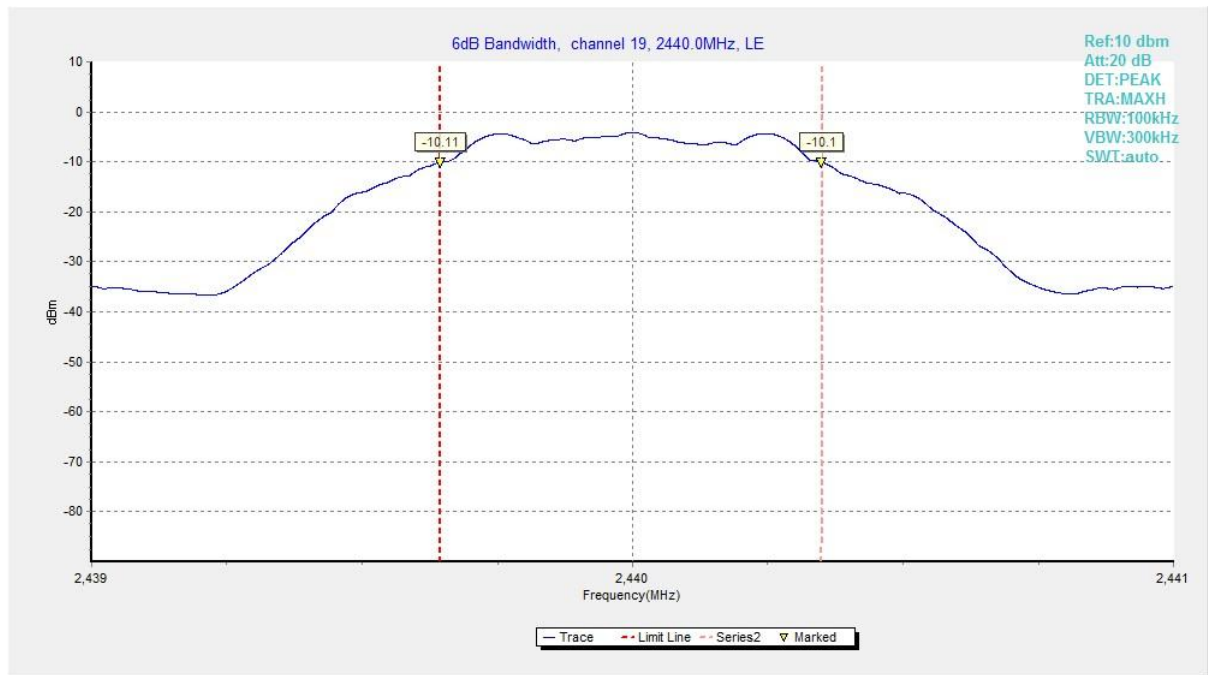
Fig.5 6dB Bandwidth (Ch 19), LE 1M
