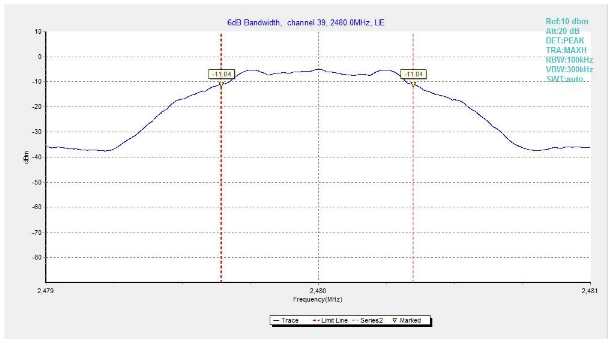
Fig.6 6dB Bandwidth (Ch 39), LE 1M
