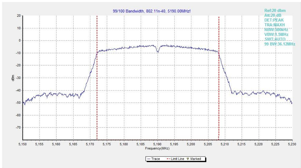
Fig. 19 99% Occupied Bandwidth (802.11n-HT40, 5190MHz)
