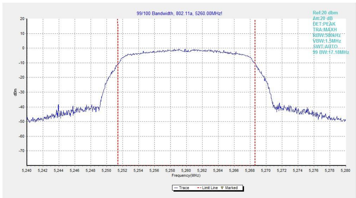
Fig. 16 99% Occupied Bandwidth (802.11a, 5260MHz)
