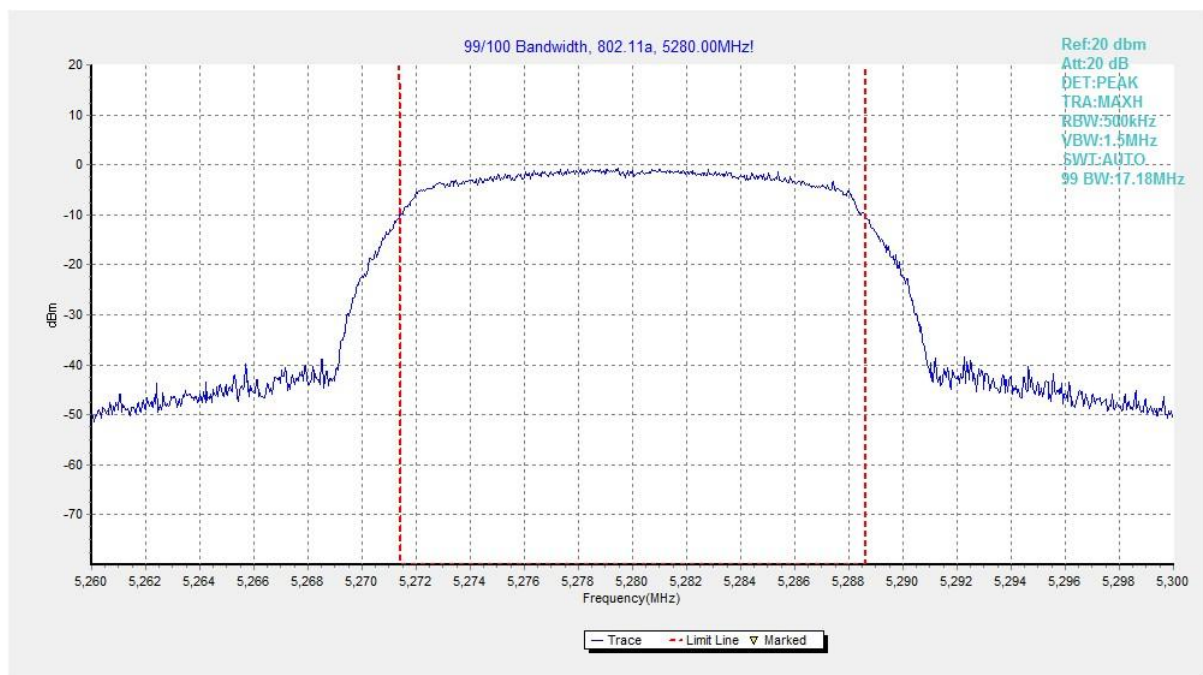
Fig. 17 99% Occupied Bandwidth (802.11a, 5280MHz)
