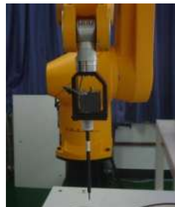
Picture C.3 E-field Probe
