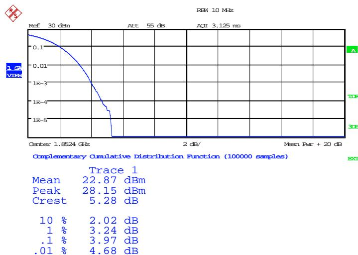
**Channel 9400- Peak-To-Average Power Ratio(PAPR)-QPSK**
