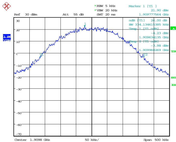
Note: Expanded measurement uncertainty is  $U = 3428\text{Hz}$ ,  $k = 2$
