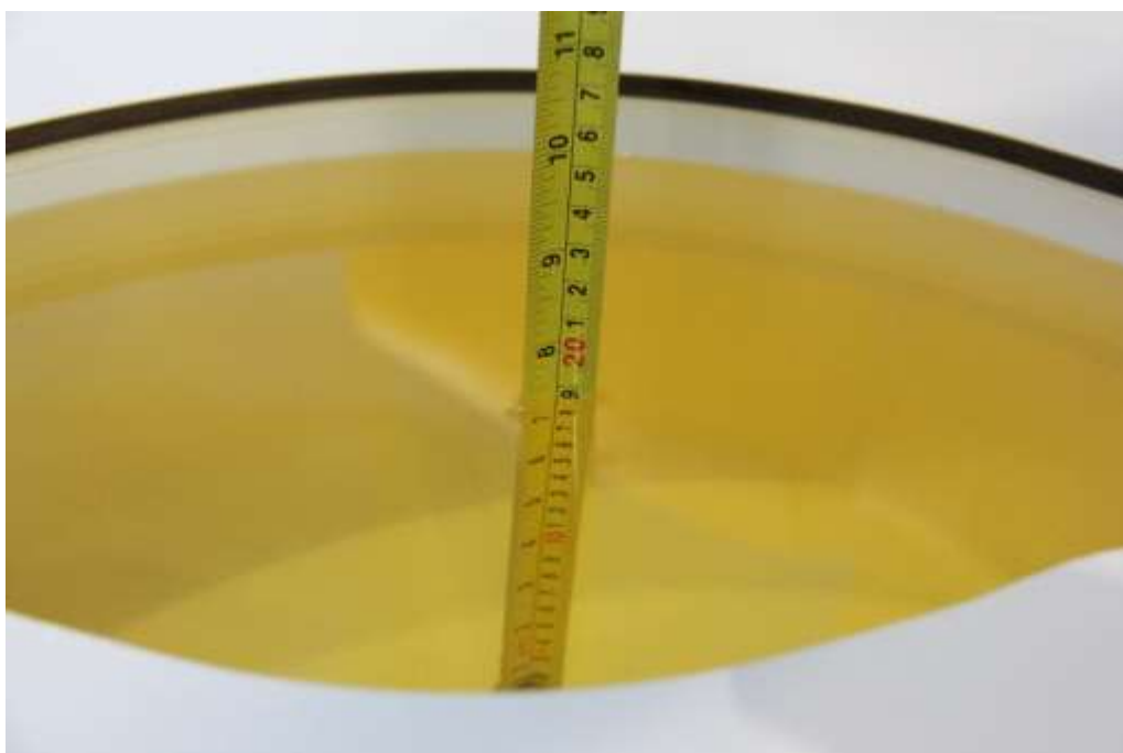
Picture 7-2: Liquid depth in the Flat Phantom (835MHz)
