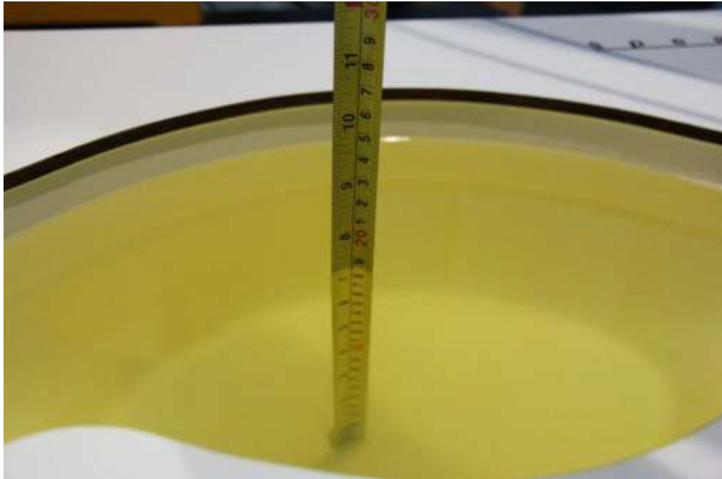
Picture 7-5: Liquid depth in the Flat Phantom(2450MHz)
