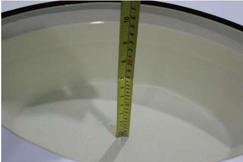
Picture 7-7: Liquid depth in the Flat Phantom(5GHz)
