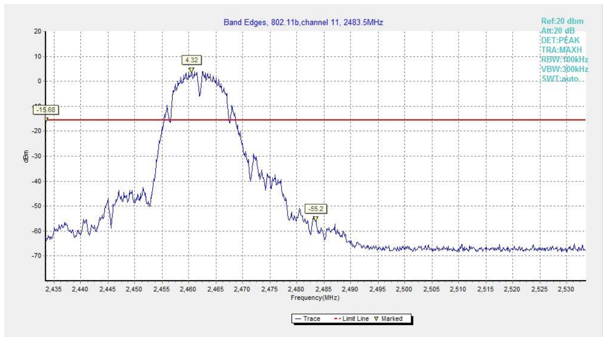
Fig.20 Band Edges (802.11b, CH 11)
