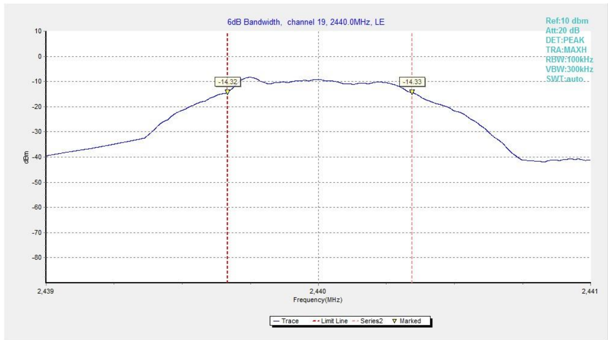
Fig.5 6dB Bandwidth (Ch 19), LE 1M
