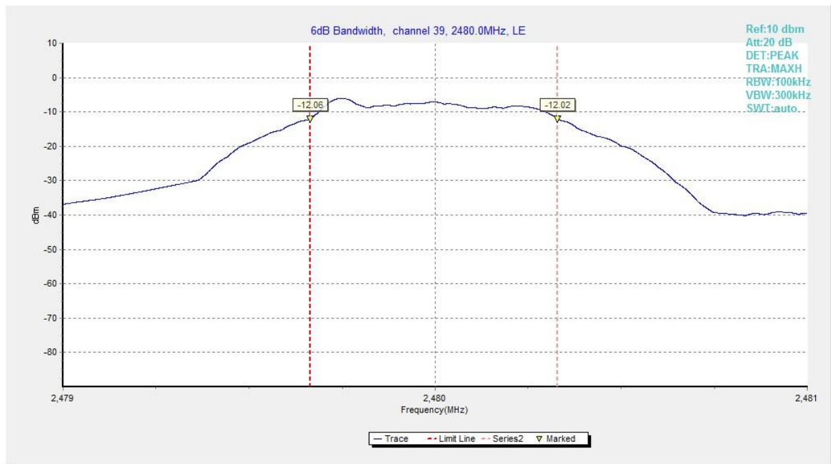
Fig.6 6dB Bandwidth (Ch 39), LE 1M
