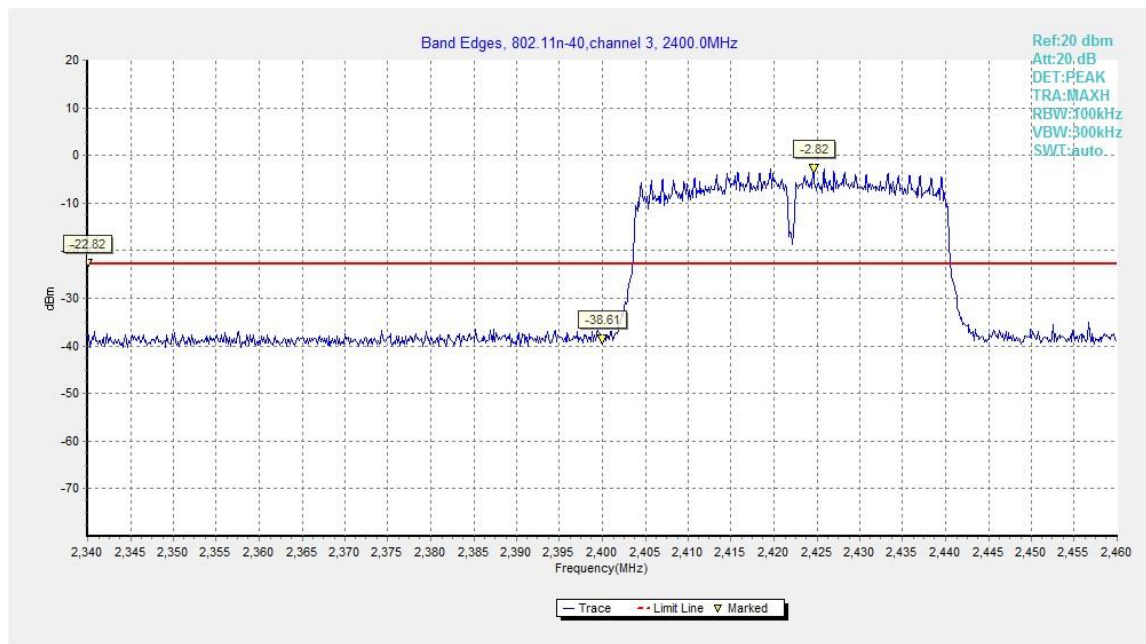
Fig.A.5.7 Band Edges (802.11n-HT40, Ch 3)
