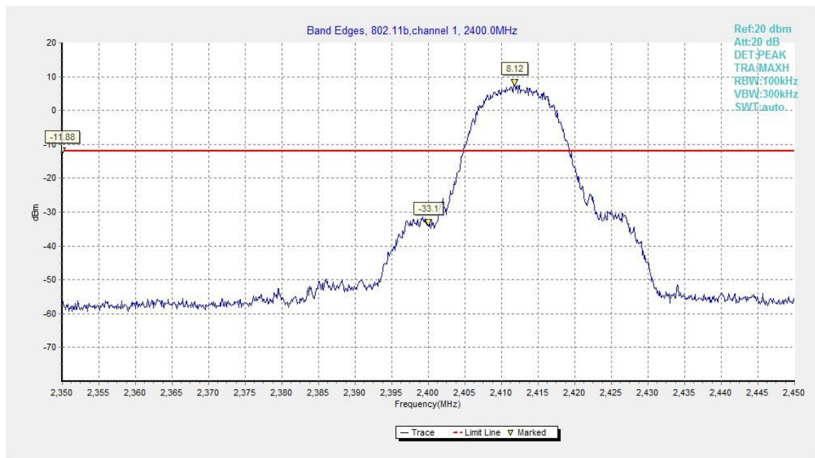
Fig.A.5.1 Band Edges (802.11b, Ch 1)
