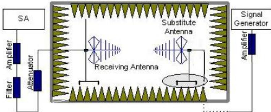
In the chamber, a substitution antenna for the frequency band of interest is placed at the
