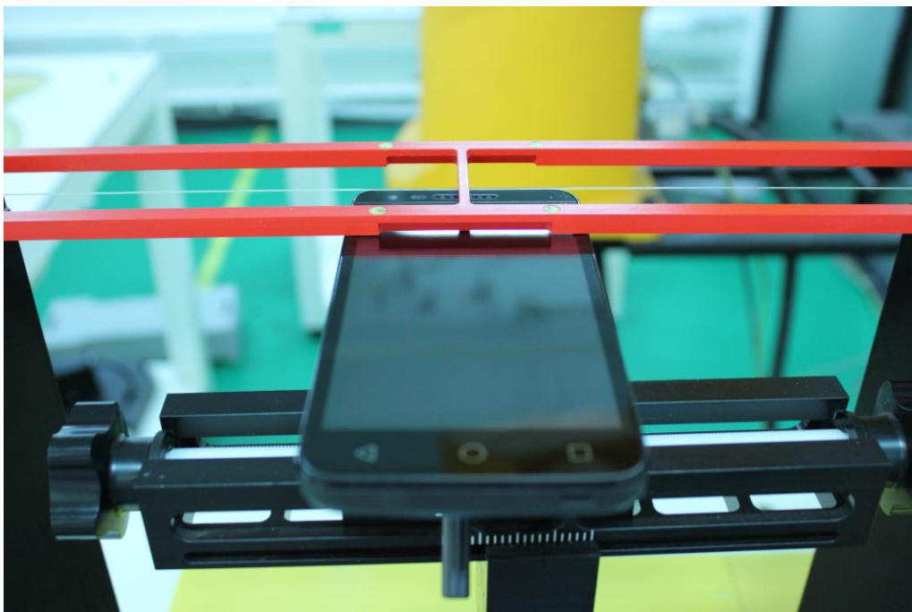
Picture 2: EUT Positioning for RF/T-coil
