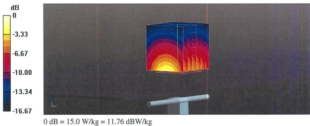
Impedance Measurement Plot for Body TSL
