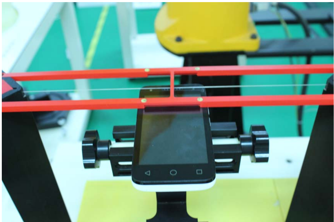
Picture 2: EUT Positioning for RF
