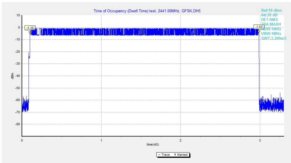
Fig.91. Time of occupancy (Dwell Time): Channel 39, Packet DH5
