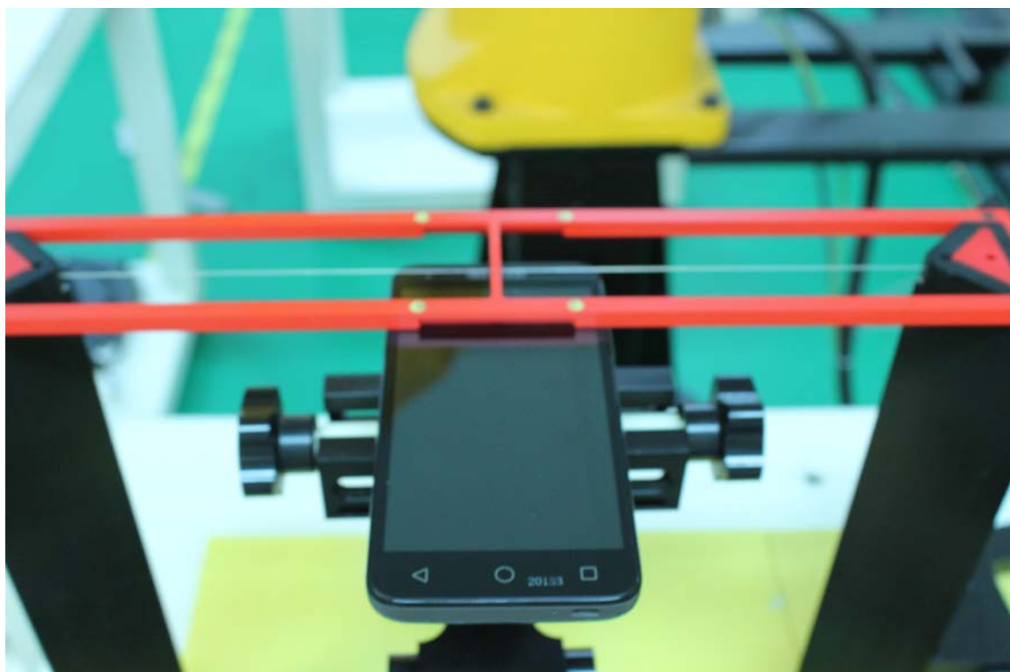
Picture 2: EUT Positioning for RF/T-coil
