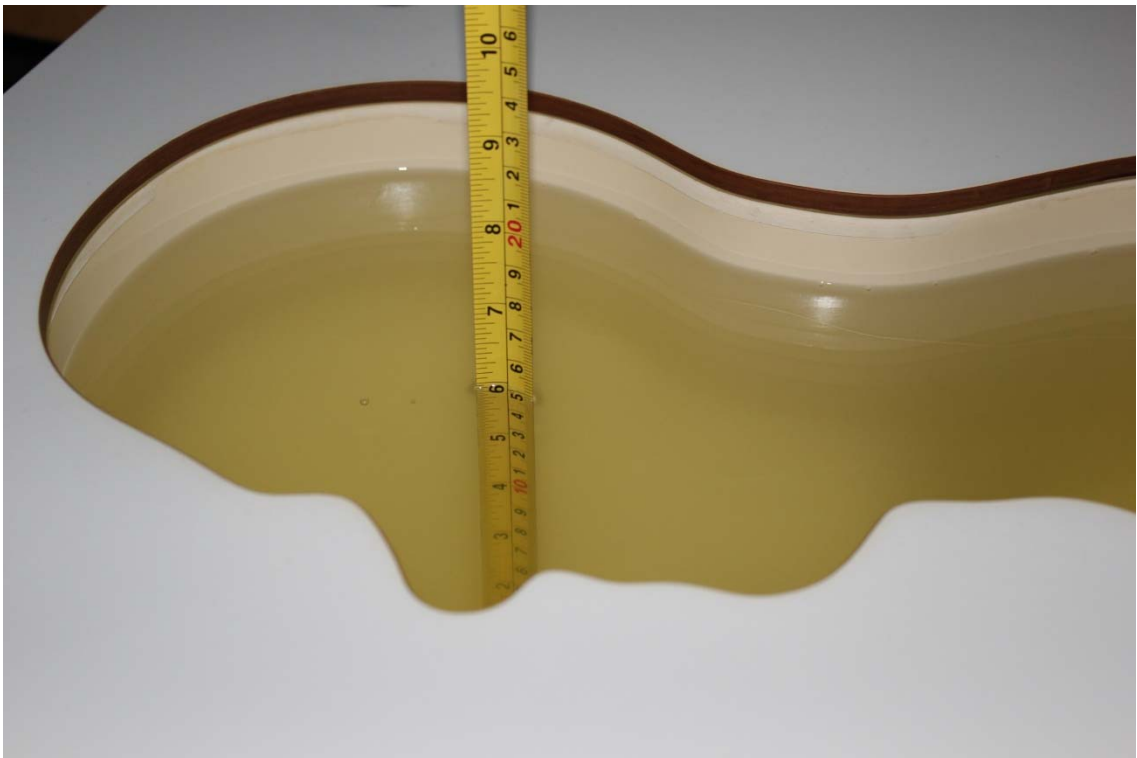
Picture 7-5 Liquid depth in the Head Phantom (1750 MHz)
