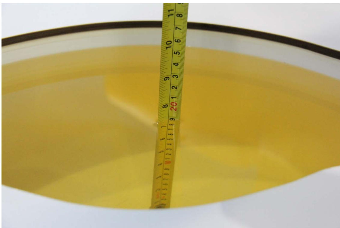
Picture 7-4 Liquid depth in the Flat Phantom (835 MHz)
