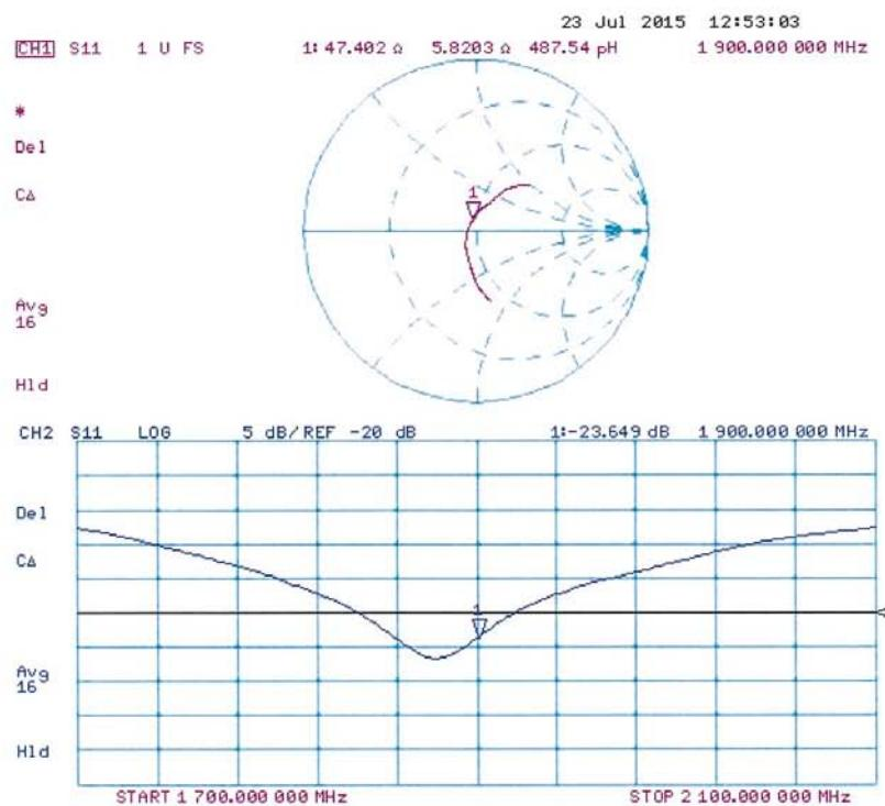
**2450 MHz Dipole Calibration Certificate for 2015**
