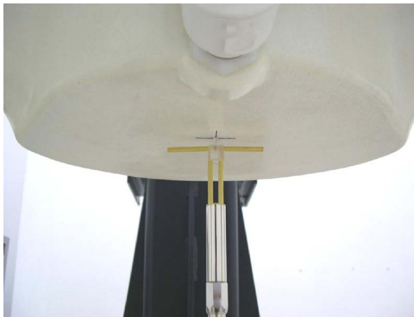
Picture 8.2 Photo of Dipole Setup
