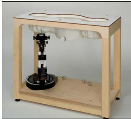
Picture C.10: SAM Twin Phantom
