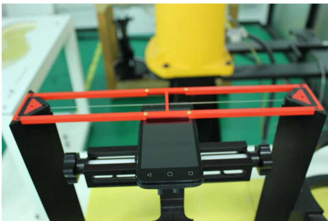
Picture 2: EUT Positioning for RF/T-coil
